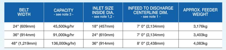
\* 1. Dimensions shown are standard. MERRICK also has manufactured many special NFPA feeders to specific dimensional requirements.
